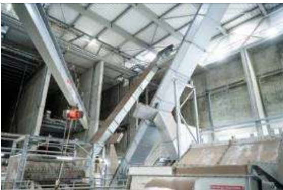
Image 2: The conveyor system then transports the material into storage boxes, en route to which an over-the-belt magnet frees the fuel from metal objects like screws and nails.
